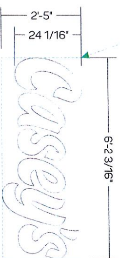
SIGN 3 CHANNEL LETTER DETAIL SCALE: 3/8" = 1'-0"
