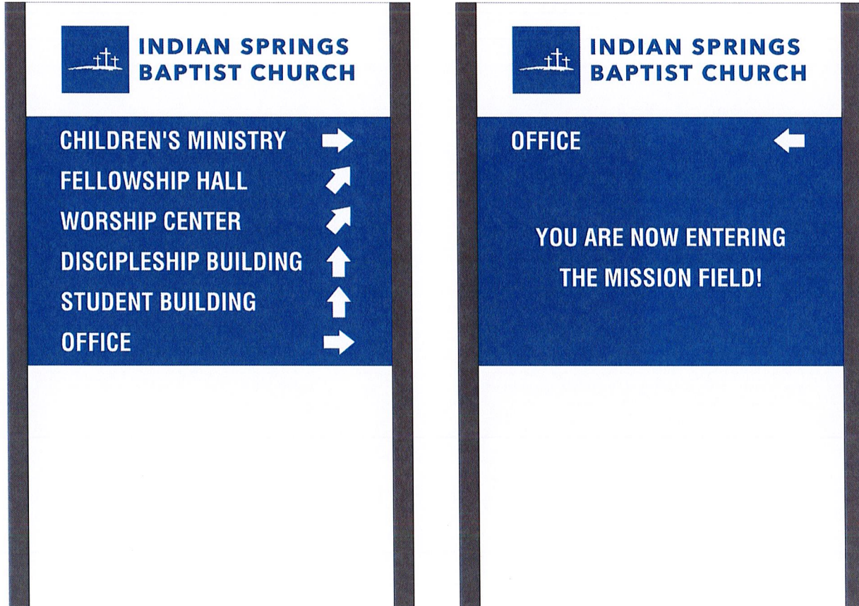
3' x 3' double sided ACM panel with applied graphics 5' overall height with posts
