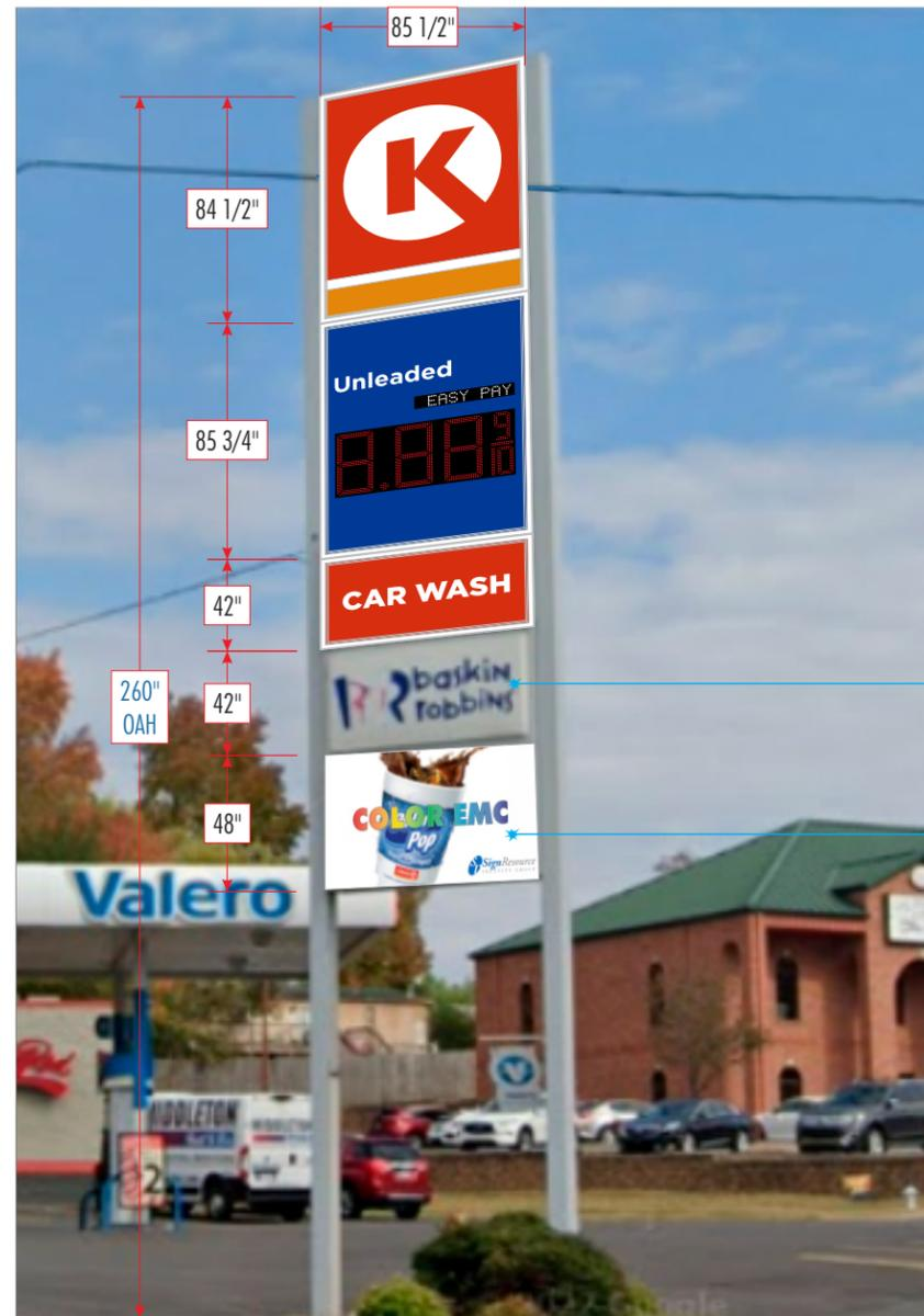
PROPOSED LEDs SIZES: NEW 24" RED ABLE 7-SEG. LEDs
