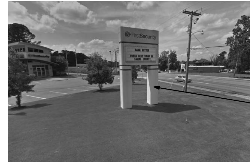
EXISTING PYLON SIGN TO BE REMOVED IN ITS ENTIRETY. EXISTING ELECTRICAL UTILITIES TO BE CAPPED AND CLEARLY MARKED FOR FUTURE USE
