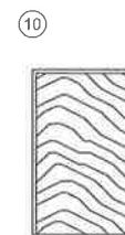
4"x7" H.M. DOOR, IN H.M. FRAME (3HR U.L. LABEL) PROVIDE PASSAGE SET
